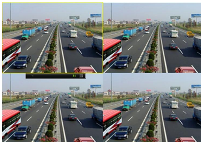
Figure 6. 1 Instant Playback Interface
